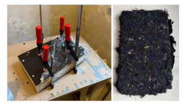
Fig. 4. Wooden mould with formed material
