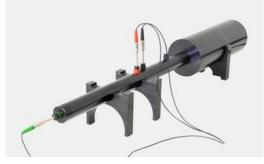
Fig. 5. AFD 1000 - sound impedance tube [15]
